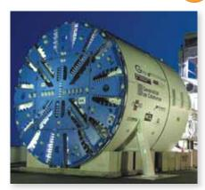
The Florida Department of Transportation plans to use a 42-foot wide tunnel boring machine to dig a 3900-foot long tunnel connecting Watson Island and Port of Miami by 2014.
